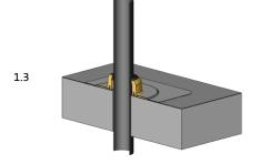
Reap the PE-pipe from the outside with lubricate and push it through the sealing ring of the installed base plate to the desired height.
