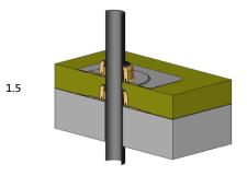
Insert the sealing ring into the base plate. Reap the built-in PE-pipe from the outside and the sealing ring from the inside with lubricant and slide the base plate from the top over the connecting pipe.
