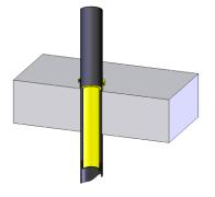
Insert the SitaVent pipe system PE-pipe into the coupler of the Sita Redevelopment adapter by using lubricate.
