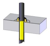
Postpone the rain deflector from above over the PE-pipe up to the base plate.
