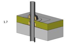
Slide the rain deflector from the top over the PE-pipe up to the base plate.
