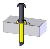
During the insertion of the rain cover or the protective grating, the fixing ring needs to be put on the installed PE-pipe and postpone the rain cover without lubricate or the protective grating with lubricant.
