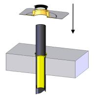
Insert the sealing ring into the SitaVent pipe system base plate. Reap the installed PE-pipe from the outside as well as the sealing ring from the inside with lubricant and postpone it from above over the connection pipe. Fix the base plate mechanically with the roof construction.
