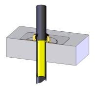
Weld or glue the roof sealing with the base plate connection sleeve.
