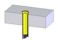
Reap the inside of the to be renovated pipe with lubricate and insert the SitaRedevelopment adapter from above.
