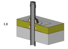
When using the rain cover or the protective grating, set the fixing ring on the installed PE-pipe and postpone the rain cover without lubricant or the protective grating with lubricant.
