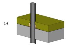
Cut the negative of the base plate into the thermal insulation and mount the thermal insulation.
