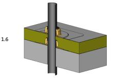
Glue or weld the roof sealing with the base plate connection sleeve.
