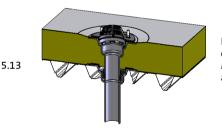
Place the dome grate in the loose flange, for conventional drainage. Mount the SitaAirstop for syphonic drainage application.
