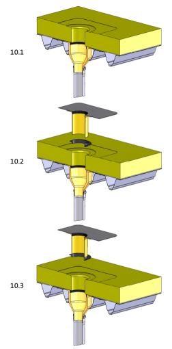
Thoroughly clean the roof outlet, extension unit, or pipe, which is to be renovated, so that a smooth surface is achieved in the area of the sealing ring.
