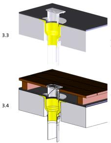
Fit the Sita terrace kit in the roof outlet or the extension element. The height of the terrace kit is adjusted through turns of the height adjustment ring, as well as through moving the housing in the height adjustment ring. The terrace kit may not be tightly connected with the outlet body in order to maintain the mobility of the parts themselves.
