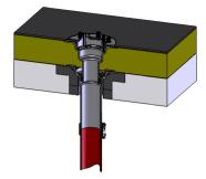
Place the SitaMulti supporting-ring with the closed side onto the cams of the SitaMulti roof outlet.
