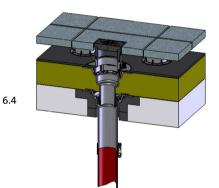
Bring a protective layer onto the sealing and work the top layer onto the grating frame.
