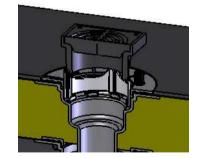
Place the housing with attached top grating of the SitaMulti grating frame onto the supportingring and adjust to the height of the top layer with the aid of the locating grooves. Height 90 mm to 130 mm.
