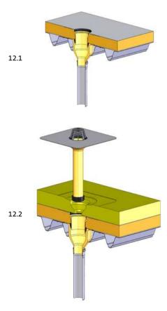
Thoroughly clean the part which needs to be renovated, so that a smooth surface is achieved in the area of the sealing ring of the renovation roof outlet.
