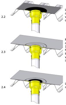
Lay the large sealing sleeve centrally on the roof outlet body. In the case of a bituminous waterproofing layer, this is to be welded directly to the outlet body.
