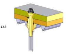
Carefully place the renovation roof outlet centrally into the part which is to be renovated and secure it mechanically. Connect the roofing material and the renovation roof outlet with the connecting sleeve, according to manufacturer's instructions. Set the dome grate in the renovation roof outlet.
