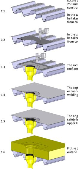
Locate the position for the roof outlet hole (ø 250 mm) at the lowest point of the roof construction.
