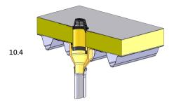
Carefully place the renovation roof outlet centrally into the part which is to be renovated and secure it mechanically. Connect the roofing material and the renovation roof outlet with the connecting sleeve, according to manufacturer's instructions. Set the dome grate in the renovation roof outlet.
