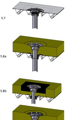
Place the angled sealing ring for backflow prevention within the outlet body, so that the upper protruding lip (between the cams) lies flush over the collar edge. Lubricate the inside of the angled sealing ring and also the extension unit with the provided lubricant.
