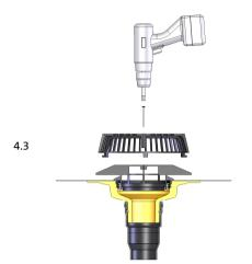
Press the stainless steel screw through the central hole of the dome grate, and screw it into the hole in the middle of the SitaAirstop.
