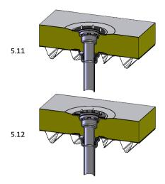
Lay the small sealing sleeve over the threaded pins onto the roofing material. Do not use the sealing sleeve in the case of a bituminous roofing material.
