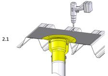
Place the screw-on-flange roof outlet or the extension unit in the existing roof construction, and screw it together with surface in the prepared vertical hole.
