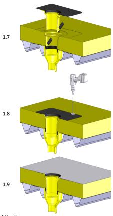
Shorten the extension element where appropriate in such a way that the outlet crosssection in the case of angled roof outlets is preserved. Apply attached lubricant medium to the lower parts of the angled sealing ring and the extension unit.
