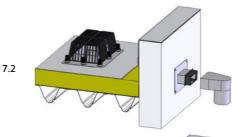
Grease the lamellar sealing from the outside and the stainless steel transition piece from the inside with lubricant.
