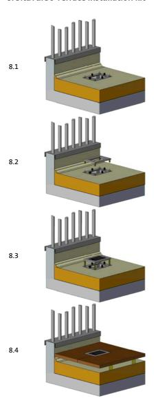
The protective caps over the nuts put on respective central or respectively remove the outer protective caps.
