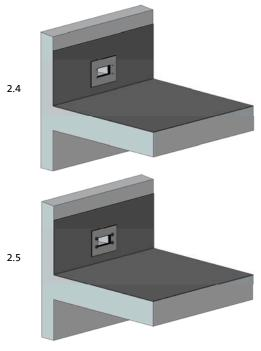
Postpone the loose-flange over the threaded pins up to the connection sleeve.
