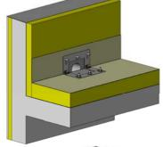
Push the washers ø36 mm over the threaded pins on the loose flange in the sealing layer. Apply the nuts and tighten alternating with a torque of max. 30 Nm.
