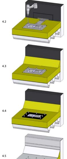
Grease the sealing of the steam vapour barrier plate and the pipe end of the SitaTurbo with lubricate.
