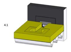
Cut out the contour of the SitaTurbo Attica outlet from the insulation.
