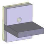
Parapet with facade breakthrough.
