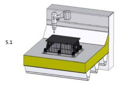
Lay the cover plate on the dome grate and align them that the holes of the cover plate are laying directly above the holes of the dome grate. Mount the cover plate with the enclosed screws.
