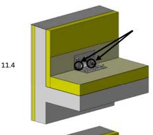
Push the bulkheads and the washer Ø 24 mm in the edge areas of the SitaRondo over the threaded pins on the loose flange. Apply the nuts and tighten alternating with a torque of max. 30 Nm.
