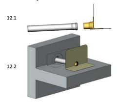
Grease the connection socket of the SitaEasy and the sealing of the coupler pipe with lubricate. Push the connection pipe on the socket of the SitaEasy.
