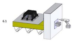
Place the cladding-cover plate over the out of the facade standing rectangular pipe of the SitaTurbo and fix it mechanically.
