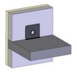
Mount the SitaSteam vapour barrier flex centrically on the facade breakthrough.
