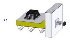
Place the lamellar sealing of the SitaTurbo outlet transition piece on the pipe end of the rectangular pipe and postpone it so much, that the stainless steel pipe lays in the three-sided Uprofile. It is important to ensure that the page without U-profile is directed downwards.
