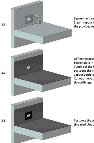
Secure the thrust-flange of the SitaTurbo Steam vapour barrier plate rigidly in front of the provided recess on the attic.
