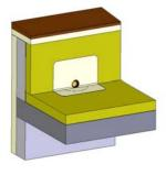
Grease the lamellar of the steam vapour barrier flex as well as the pipe of the component with lubricate. Push the pipe through the lamellar of the steam vapour barrier flex and insert the component to the determined position into the flat roof construction. The component needs to be fixed mechanically.
