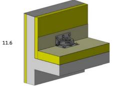
Put the dome grate with the angle bracket on the middle threaded pin in the parapet layer. Push the washer ø36 mm over the threaded pins on the loose flange or respectively angle bracket. Apply the nuts and tighten alternating with a torque of max. 30 Nm.
