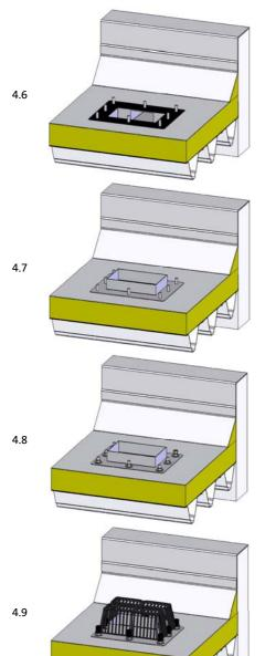
Lay the small rubber sealing sleeve over the threaded pins on the roof track. In case of a bituminous seal a sealing sleeve is not applicable.
