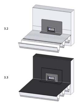
Mount the SitaTurbo Steam vapour barrier flex in front of the parapet recess.
