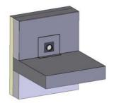
Glue the vapour barrier on the adhesive flange of the flexible steam vapour barrier.
