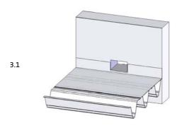
Roof construction with identified recess in the parapet.
