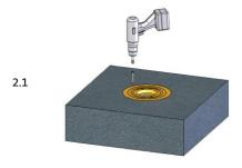
Put the SitaCompact screw-on-flange balcony outlet or the extension unit in the existing roof construction and screw it through the polyurethane flange, outside of the flange, to the ground.
